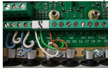
**TERMINALS 9, 10, 11 BETWEEN FLOW SENSOR AND INTEGRATOR MUST ALWAYS BE SEALED WITH THE SUPPLIED USER SEAL AFTER INSTALLATION!**
